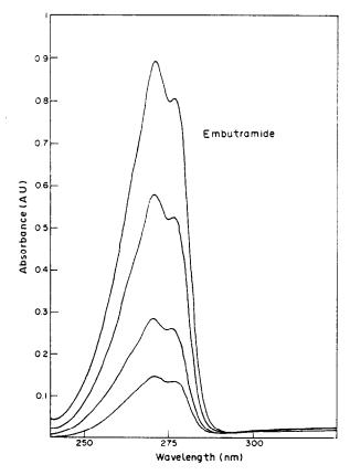
Figure 1 UV spectra of embutramide calibration standards.
